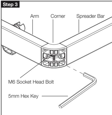
3. Secure by tightening the M6 Socket head bolts using 5mm Hex Key.
