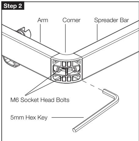
**2.** Loosen the M6 Socket Head Bolts using 5mm Hex Key and remove corner from Arm and Spreader Bar. Discard old Corner.
