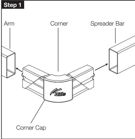
1. Insert Corner into Arm and Spreader Bar.
