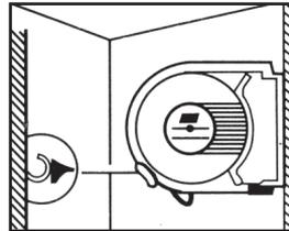
2. Once free end is fastened over retention hook, pull the line taut from the reel end. Loop line twice around the locking cleat at the
